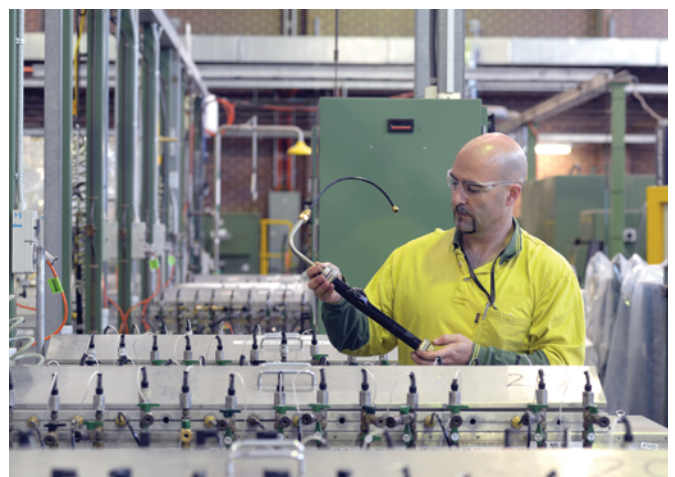
Pressure data collection at elevated temperatures in the Qenos Technical Centre, Altona
