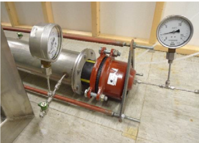
Figure 2. Permeation experimental setup in which the PE pipe (black with yellow stripes) is capped and pressurised whilst permeation is measured by gas chromatography in a stainless steel jacket pipe.
